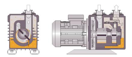
The machine works on the two-stage rotary vane principle.
